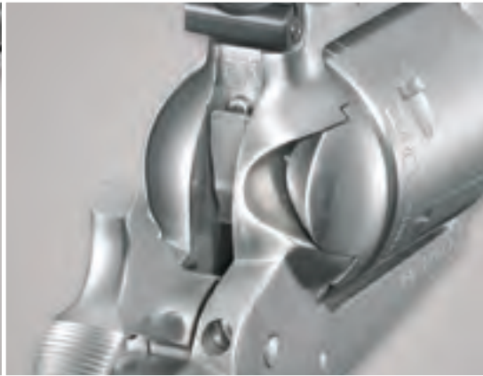
Patented Ruger® Transfer Bar Mechanism
