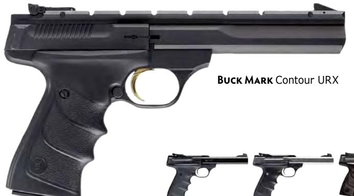
Browning Buck Mark rim-fire pistols are very highly valued due to their quality, reliability and accuracy. These pistols have a receiver made from a single aluminium block machined using numerical control. The barrel is machined in a single top-quality steel block and the chamber is hand-bored for guaranteeing optimal accuracy. Every Buck Mark pistol has fully adjustable sights.
