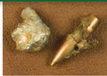
Both of these projectiles were fired at a Russian brown bear from less than 20 yards. At left is the remnant of a 16 gauge shotgun slug of inferior alloy; at right, a 7.62 mm FMJ rifle bullet. Both penetrated less than three inches beyond the great beast's skin. The slug hit the bear's shoulder and stopped cold; the 7.62 bullet was deflected sideways by a rib. Fortunately for all parties involved, the primary hunter was using a higher quality projectile. This demonstrates the inherent dangers of a projectile that does not penetrate adequately.
